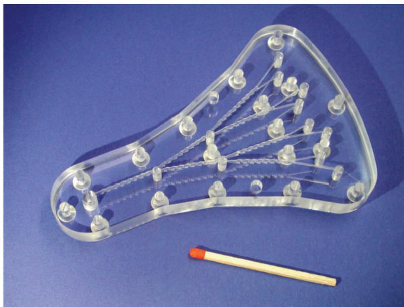
**Figure 1** This system is grouping microreactors in line and in parallel, in order to materialize physical systems described by CDS formalism. Eight inlets can drive gases, liquids and solids into channels where they are dispersed. The prototype has been designed in collaboration with the Institut für Mikromechanik Mainz (IMM), and constructed by Volker Hessel and his team at IMM.
